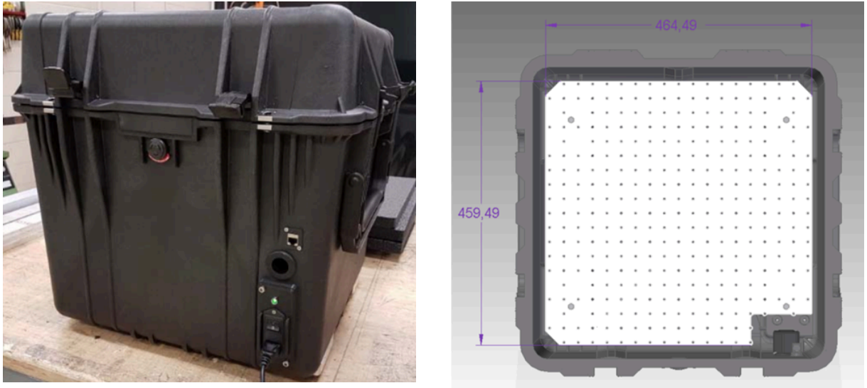
Figure 2.1: (a) Pelican case exterior with modifications (bottom-right corner) (b) Pelican case interior mounting plate with dimensions 459.49 x 464.49 mm.
